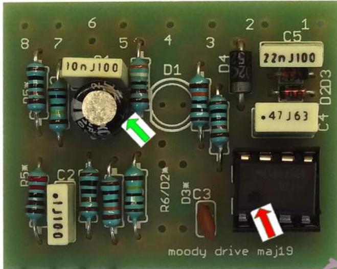
Image 1. Location of the components on the PCB.
