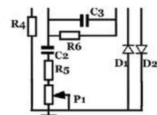
Image 5. Alternative way of adjusting gain.
