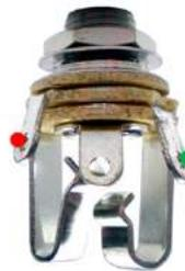
The **Input jack** is stereo. It has three pins: "tip", "ring" and "ground". The image shows tip marked with a red dot and ring marked with a green dot. **Do not mix them up!**
