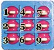
The **Footswitch** S1 has 9 pins. We assign them numbers, 1 through 9. **To get the switching right, mount S1 with its pins in parallel with the short sides of the box** (see images 2 and 3). It is ok to turn it 180 degrees with respect to this direction (but not 90 degrees). **Avoid overheating the pins!**
