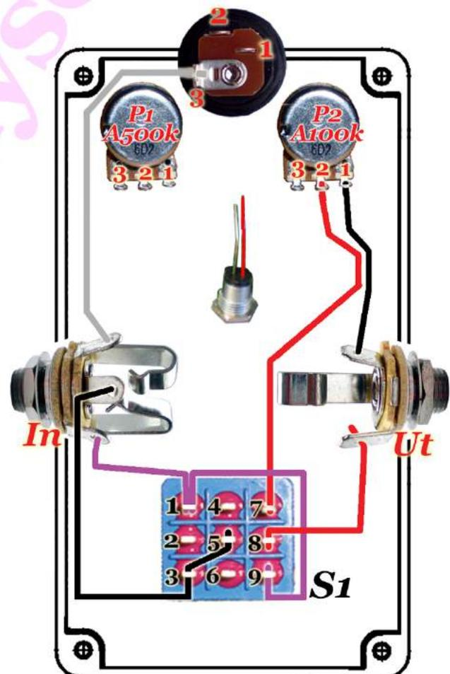
Image 2. S1's pins shall be in parallel with the short sides of the box.
