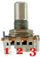
A **Potentiometer** has three solder lugs: 1, 2 and 3. Its value is written next to its shaft. **P1 and P2 have different values - do not mix them up!**
