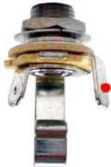
The **Output jack** is mono. and it has two solder lugs, which we call "tip" and "ground". Tip conducts with the "arm" of the jack and it is marked with a red dot in the image to the left.
