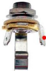
The **Output Jack**, "UT," is a mono jack and it has two solder lugs, which we call "tip" and "ground". Tip conducts with the "arm" of the jack and it is marked with a red dot in the image to the left.
