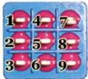
The **Footswitch S1** has 9 pins. We assign them numbers, 1 through 9. **To get the switching right, mount S1 with its pins in parallel with the short sides of the box** (see image 2). It is ok to turn it 180 degrees with respect to this direction (but not 90 degrees).
