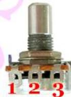
A **Potentiometer** has three solder lugs: 1, 2 and 3. Its value is written next to its shaft. **P1, P2 and P3 have different values!**
